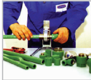
Heat Pipe and fitting at same time
